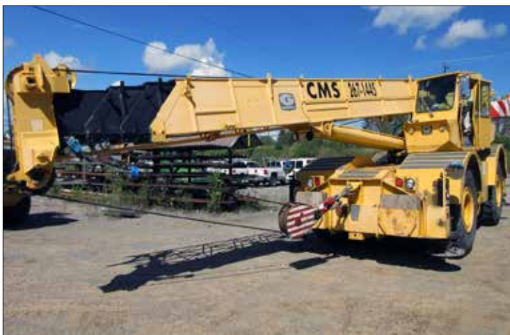
GROVE 35-Ton Rough Terrain Crane, Mdl. RT65S
