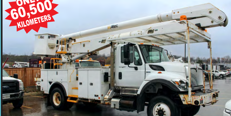
Altec AA755MH 55' Platform Height 700lbs Cap Articulating Bucket Mounted on 2012 International WorkStar 7300 7.6L Diesel 4x4
