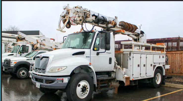
Altec DM47BC Digger Derrick w/ Winch & Hydraulic Outriggers Mounted on 2013 International DuraStar 4400 MaxxForce 7.6L Diesel
