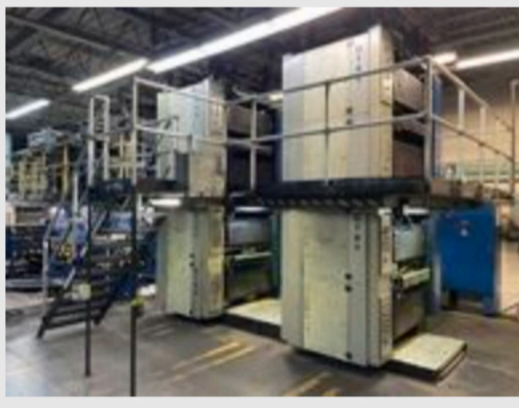
Global 35" Press, 22.75" Cutoff, 18 Units Model G145: (4) 4 high, (1) 2 high, (2) folders, (2) JTI double (1) JTI single splicers, Quadtech registration, Perretta Graphics ink control
