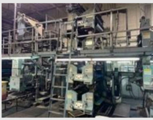
Goss 34" Press 22.75" Cutoff, 28 Units: (5) 4 high, (4) 2 high, (3) Folders, (6) Enkel double splicers
