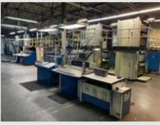
Global 35" Press, 22.75" Cutoff, 18 Units Model G145: (4) 4 high, (1) 2 high, (2) folders, (2) JTI double (1) JTI single splicers, Quadtech registration, Perretta Graphics ink control
