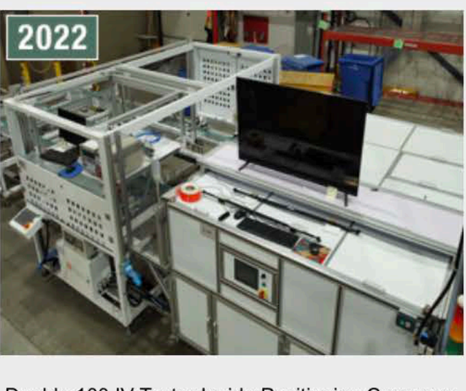
Double 100 IV Tester Inside Positioning Conveyor, Model DB100-IVDX03
